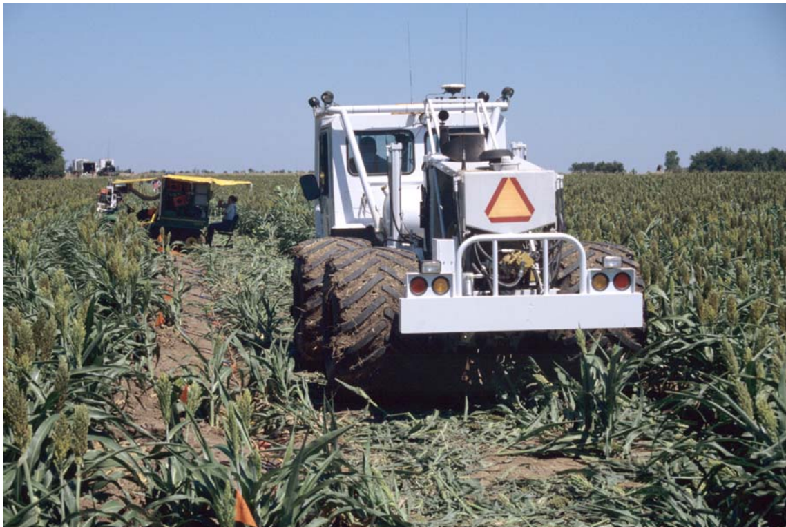
Figure 5: Collecting data in a milo field using a 240-channel seismograph and the custom-made "MiniVibe"
