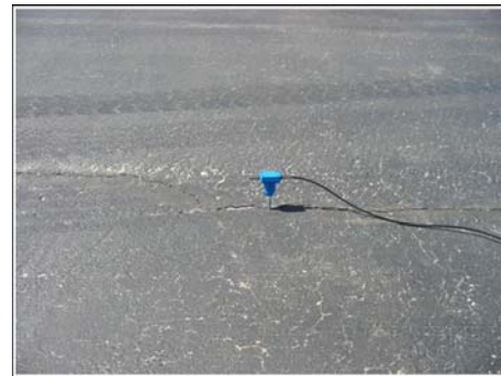
Figure 5. View of typical geophone secured into pavement prior to surveying.
