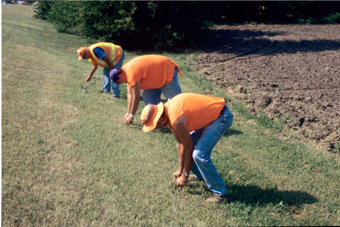
Figure 4: Placing geophones on the first day of the survey
