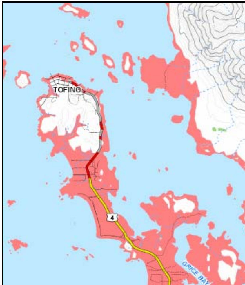
Figure 2: Provincial Highway segments susceptible to impact by tsunami from large magnitude earthquake near Tofino, BC.
