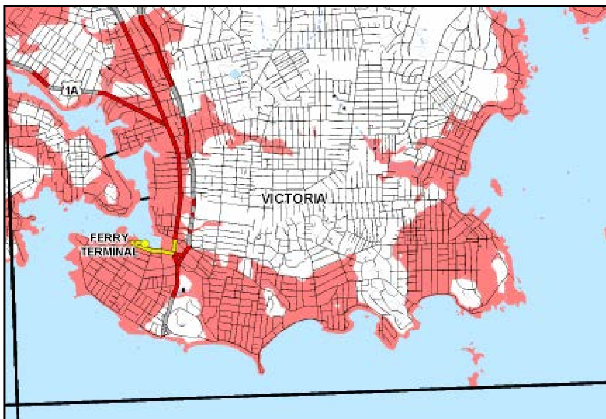
Figure 5: Provincial Highway segments susceptible to impact by tsunami from large magnitude earthquake in Victoria, BC.
