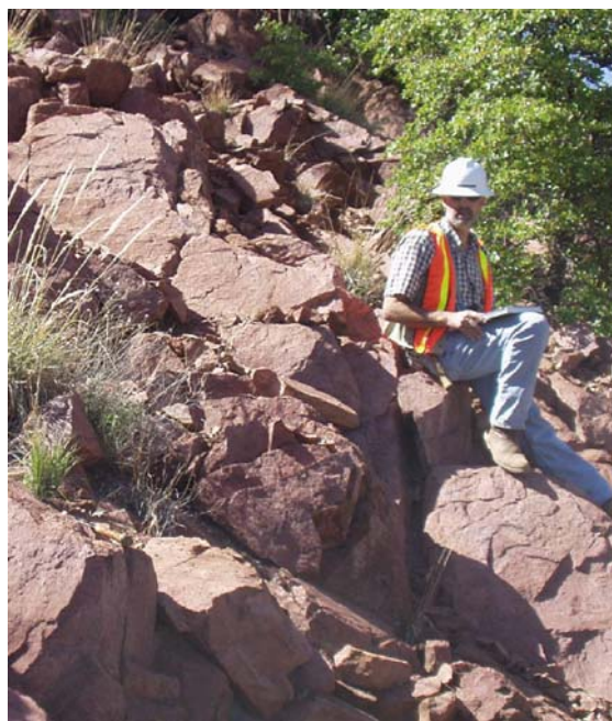
Photograph 5 – Bedrock outcrop above new US 191 alignment near middle of project. Note unfavorably dipping rock structure.
