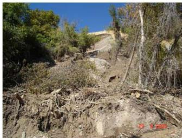
Figure 3: The slide configuration after the second movement (September 26).
