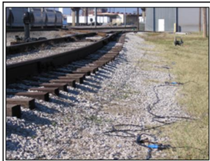
Figure 4. View along ReMi Line 1 showing 20-foot geophone spacings.
