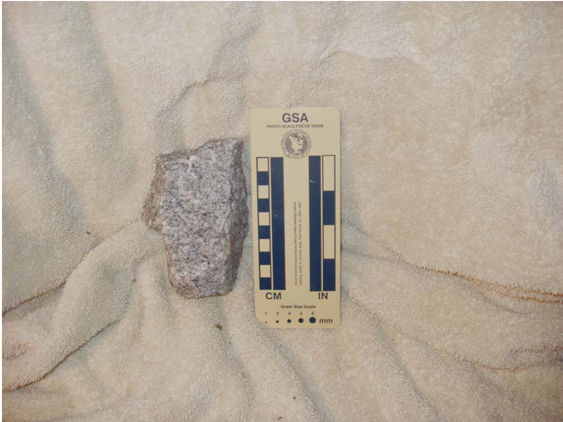
Figure 8. Quartz monzonite from the Burkeville Pluton and Luck Stone, Incorporated's facility in Burkeville. Quartz monzonite is marginal to granite, and often possesses favorable characteristics for use as aggregate in asphalt.
