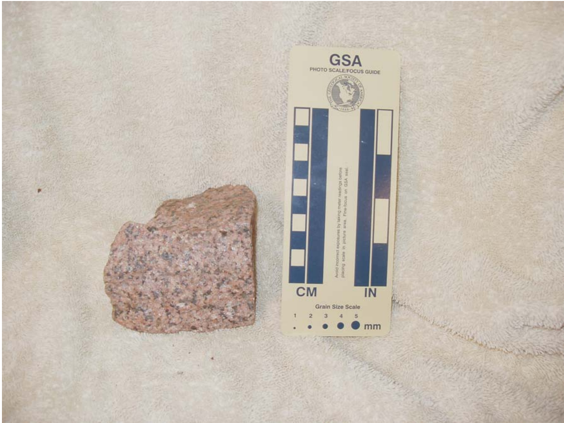
Figure 5. Tishomingo Granite from Meridian Aggregates' Snyder facility, southern Oklahoma. Macroscopically, the graphic texture of the granite is readily visible.
