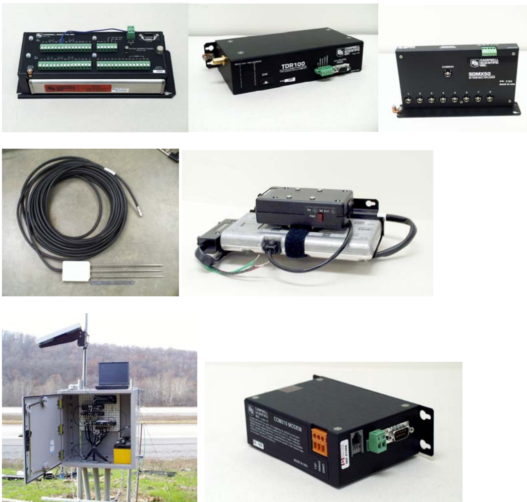
Figure 2. TDR hardware used in this study; Clockwise from top left, 16 channel data logger, cable tester, multiplexer, , analog cell phone, modem, complete field installation, TDR moisture probe.
