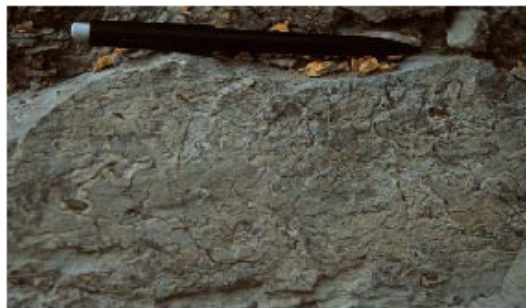
Figure 5. Photo of a bed of phylloid algal wackestone with completely disseminated argillaceous material throughout its thickness. This form of clay is recognized by the bluish-gray color it imparts to the rock. Due to the disseminated nature of the clay, it will become part of the aggregate following crushing of the rock.
