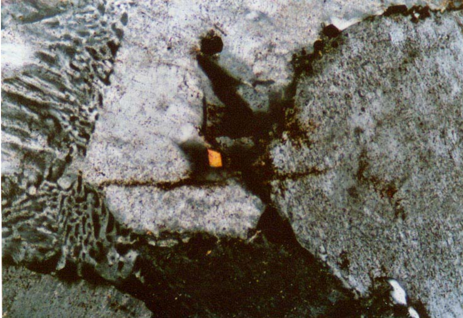
Figure 12. Quadrilateral sphene (titanite) grain as accessory mineral enclosed by quartz in graphic granite. Note micrographic texture on left side of photomicrograph. Granite from Meridian Aggregates Long Mountain (Snyder) facility, Jackson County, Oklahoma. Crossed polars, 100X.
