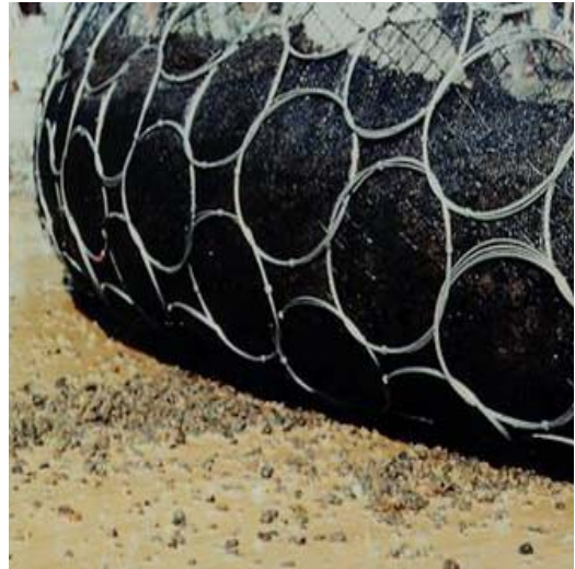
Figure 3 - Debris in Ring Nets During Test
