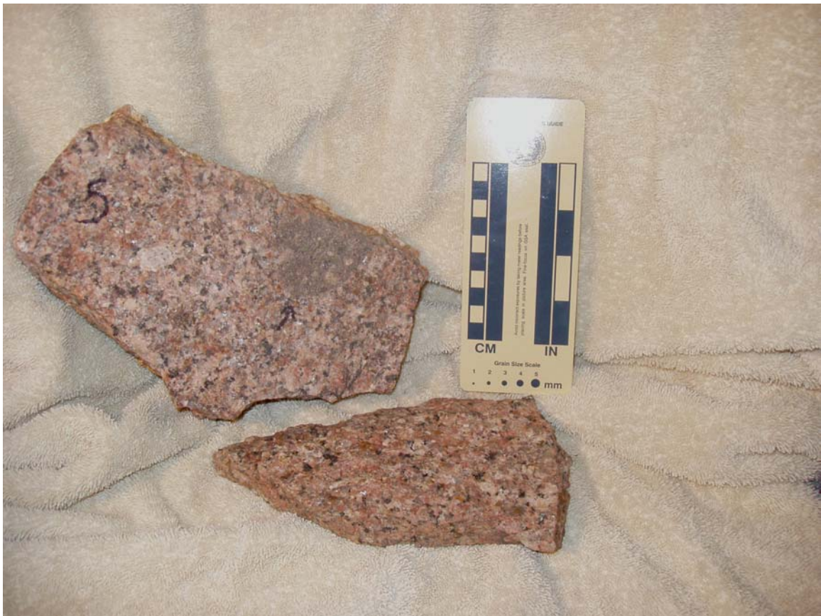
Figure 2. Butler Hill Granite from southeast Missouri. This granite is similar to Graniteville, except that it possesses muscovite mica and has a peculiar type of texture, known as 'rapakivi'. In this texture, rims of orthoclase surround larger grains and phenocrysts of plagioclase. The reverse is referred to, rather unimaginatively, as 'anti-rapakivi'. Butler Hill Granite possesses both rapakivi and anti-rapakivi textures. The upper sample shown here also possesses a large ragged-edged xenolith of unknown composition.
