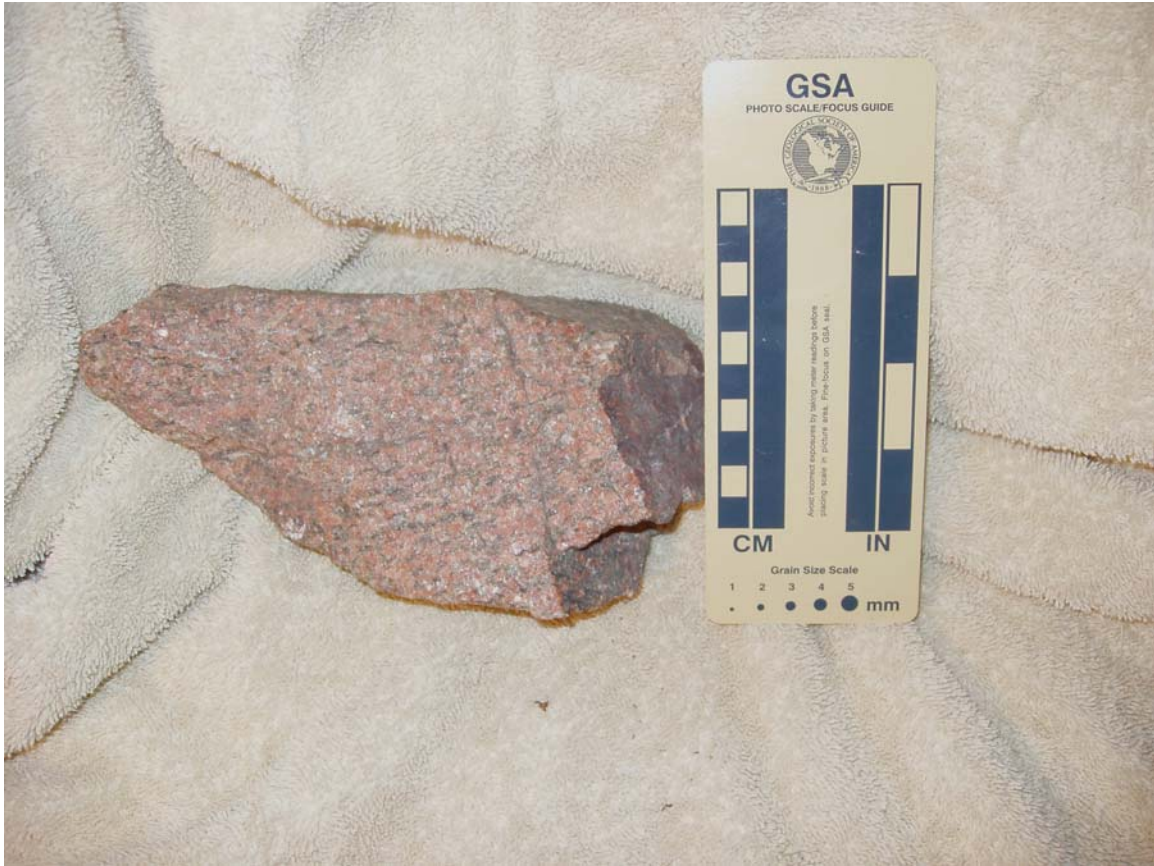
Figure 7. Cranberry Gneiss from eastern Tennessee. This rock, though it contains orthoclase, quartz, and plagioclase in similar proportions to granite, may not be an ideal aggregate stone for paving purposes. It is a metamorphic rock which has undergone stress. This stress may render it susceptible to alkali-silica reactivity (ASR) in a concrete pavement. Additionally, the stone possesses foliation planes that are markedly prominent enough to where it may increase the percentage of flattened and elongated particles in a crushed stone product. This would render it largely unsuitable for asphalt paving stone unless a sufficiently small gradation was found to decrease the overall percentage of flattened and elongated particles in an asphalt pavement. Gneisses can form from a variety of igneous and sedimentary rocks, thus, it is not always clear what rock is the precursor to the final metamorphic gneiss. Impurities in a variety of forms may also be present, as is the norm for many metamorphic rocks.
