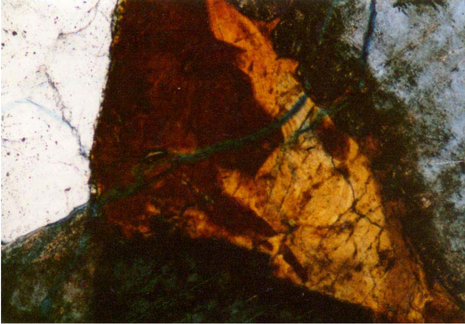
Figure 10. Undulatory extinction in pleochroic biotite grain also indicative of stress from dike injection of basalt. Troy Granite, Meridian Aggregates' Mill Creek Quarry. Johnson County, Oklahoma. Crossed polars, 100X.
