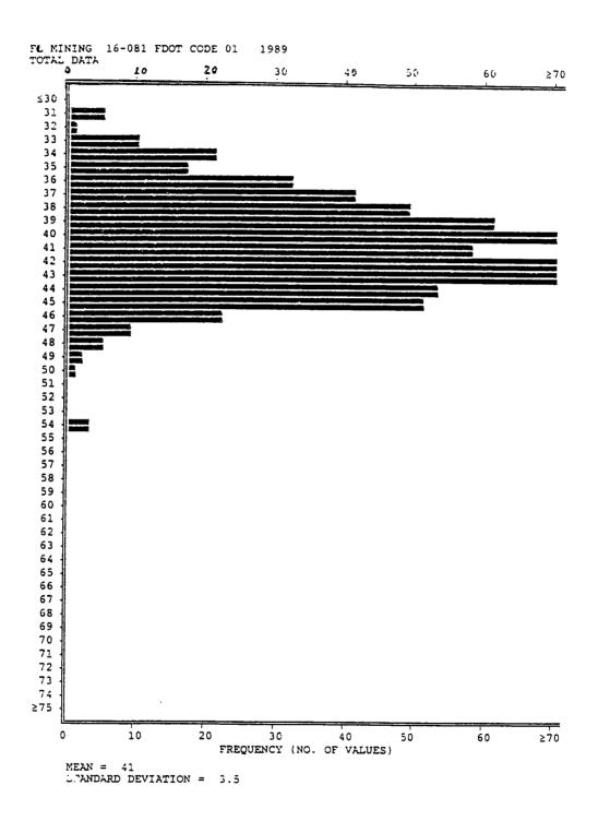
Figure 4. Histogram of Distribution of Data for Number 30 Sieve for Silica Sand.
