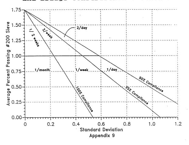
Figure 8. Sampling and Testing Frequency Chart for a Single-Ended Specification.
