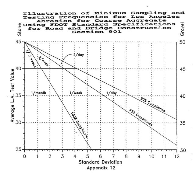
Figure 10. Sampling and Testing Frequency Chart for L. A. Abrasion of Different Types of Aggregate.
