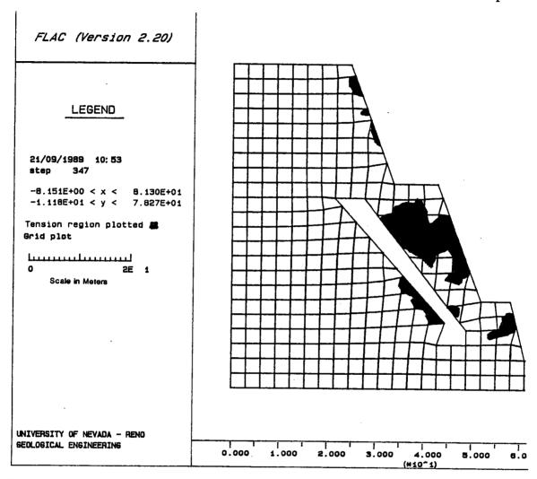
Figure 7. Tensional stress development induced by underground workings.
