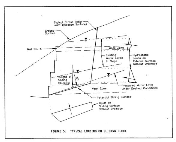
The forces opposing sliding are provided by the frictional strength of the material forming the base of the block and the force provided by the tie-backs. The
