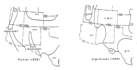
FIG. 2-Seismic risk maps. Intensities according to Modified Mercalli Intensity Scale of 1931.
