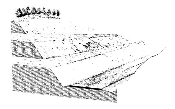
Figure 20. This block diagram illustrates the slope flattening concept (to reduce rockfall) as applied along I-40 in Cumberland County.
