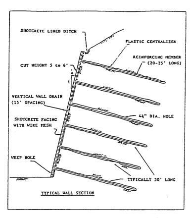
Figure 5. Details of Cumberland Gap Soil Nailing
