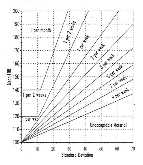
Figure 12. Sampling and Testing Frequency Chart for Limerock Bearing Ratio Test in Base Materials.
