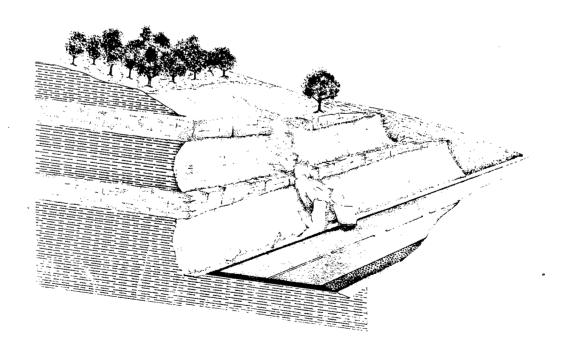
Figure 19. This diagram shows the typical rock slope condition along I-40 in Cumberland County prior to the remedial project.
