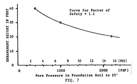
Long term stability of the 40 foot embankment is estimated to have a Factor of Safety of 1.78.
