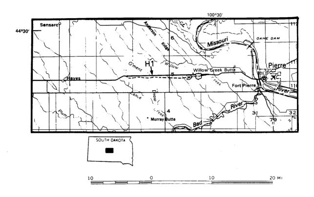
FIGURE 1. Map showing location of fault-related highway damage in a cut along U.S. Highway 14 (site H1) within the Stanley County, S.Dak., study area. The abandoned section of U.S. Highway 14 is shown by a dashed line.
