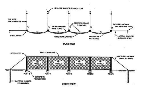
FIGURE 1. PLAN VIEW AND FRONT VIEW OF BRUGG ROCK NET
