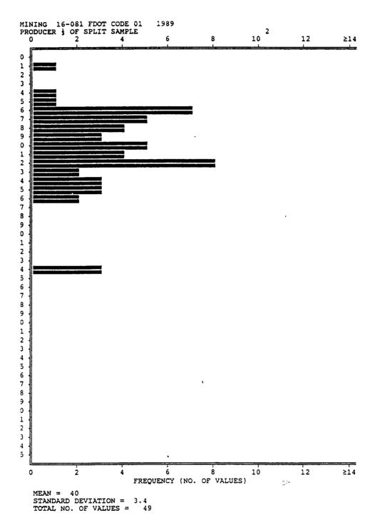
Figure 5. Histogram on Number 30 Sieve for Silica Sand(Producer Half of Split Sample).
