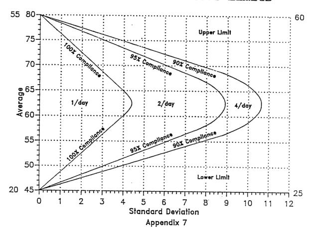
Figure 7. Sampling and Testing Frequency Chart for a Double-Ended Specification.
