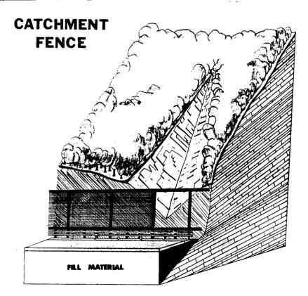
Figure 5. Wire meshing and catchment fences were two types of protection devices employed in the rockfall remedial project.
