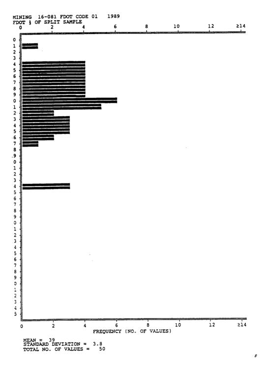
Figure 6. Histogram on Number 30 Sieve for Silica Sand(FDOT Half of Split Sample).
