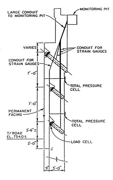
Figure 3. Instrumentation Details, Ramp Q Abutment
