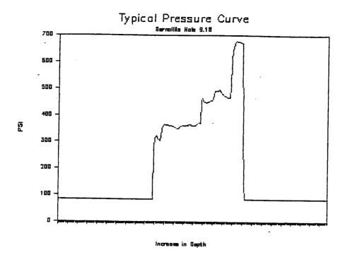
Cone Resistance at 365.5 psi Friction Resistance at 466.7 psi
