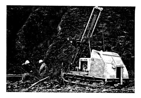
Figure 3. Bombardier Mounted Drill
