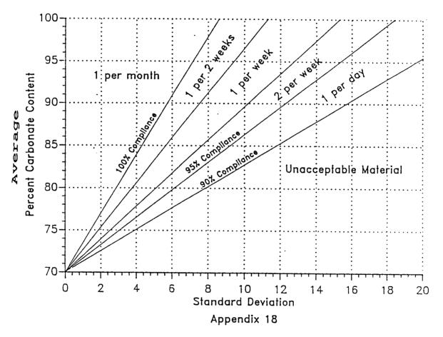
Figure 11. Sampling and Testing Frequency Chart for Carbonate Content in Limerock Base Material.
