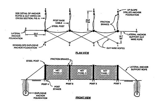
FIGURE 3. PLAN VIEW AND FRONT VIEW OF THE INDUSTRIAL ENTERPRISE ROCK NET CONSTRUCTED FOR THE INITIAL FIELD TESTING
