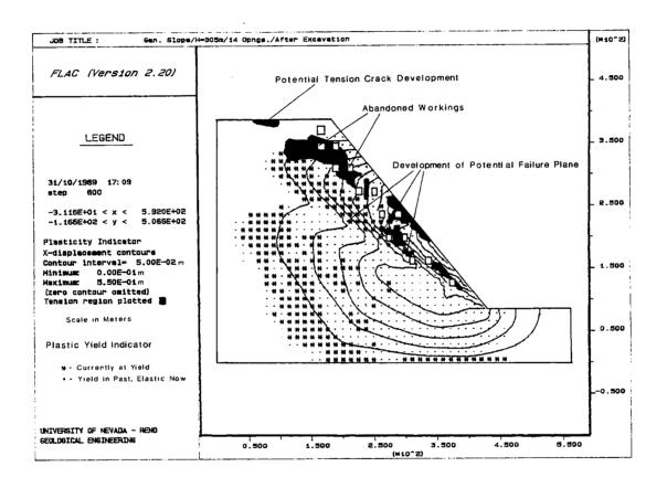
Figure 6. Finite difference model showing yielding joints and tension zones.
