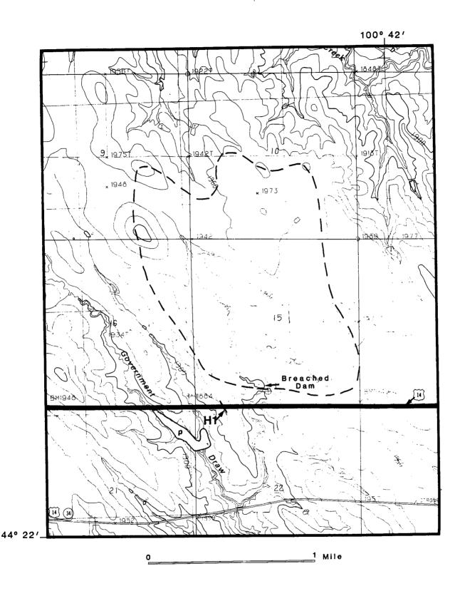
FIGURE 5. Index map showing the fault exposure at site H1 on new section of U.S. Highway 14 (solid line), the new (since 1982) stock dam (P), and the enlarged drainage area of the tributary to Government Draw (dashed line) developed above the breached dam (arrow). The culvert and gabion affected by upstream migration of a knickpoint in the tributary are shown in greater detail in figure 2.
