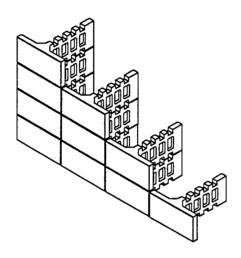
Fig. 1. T-WALL<sup>TM</sup> RETAINING WALL (A patented system)
