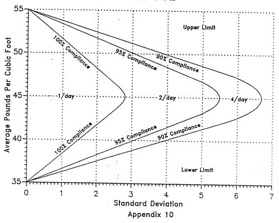
Figure 9. Sampling and Testing Frequency Chart for Specialized Lightweight Aggregate.
