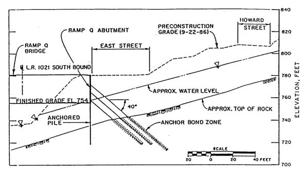
Figure 2. Schematic Cross-Section, Ramp Q Abutment
