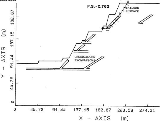
Figure 5. Bench instability failure surface, due to underground workings.
