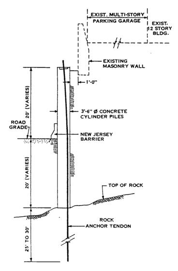
Figure 1. Post-Tensioned Caisson Retaining Wall
