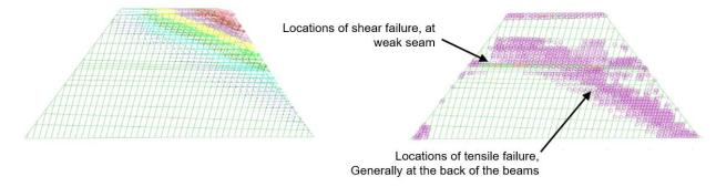
Figure 11 – Flexural toppling displacement vectors and failure locations (Station 194+00, deterministic analysis, 1.2 strength reduction factor).
