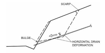
Figure 9 – Illustration of potential damage in cut sections
