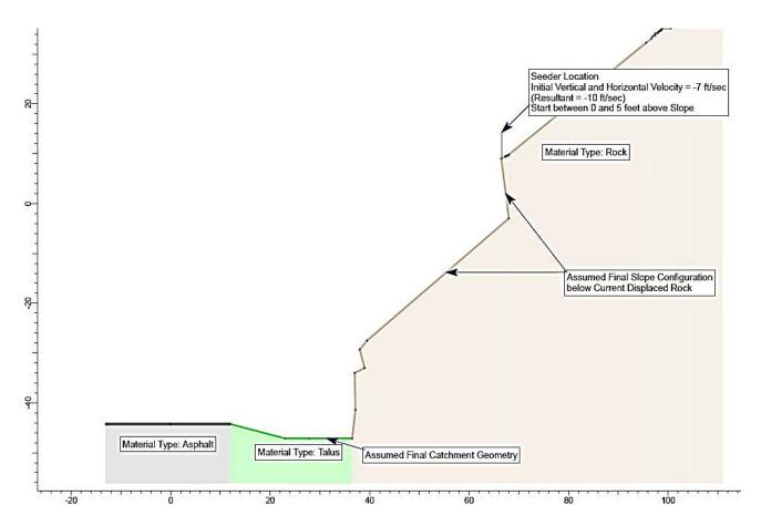
Figure 12 – Final Slope Configuration for Catchment Performance Evaluation
