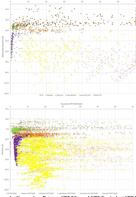
Figure 4 – Comparison Between SPT N1<sub>60</sub> and CPT Equivalent SPT N1<sub>60</sub>
