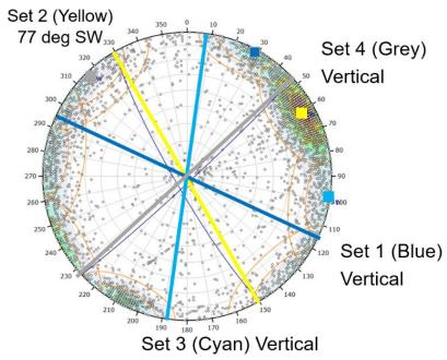
Figure 5 – Lower hemisphere stereonet of joint set orientations for the isthmus rocks.
