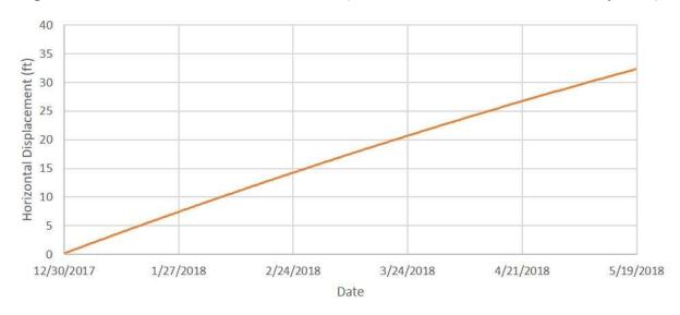
Figure 7 – Landslide Horizontal Movement (robotic total station, January to May 2018)
