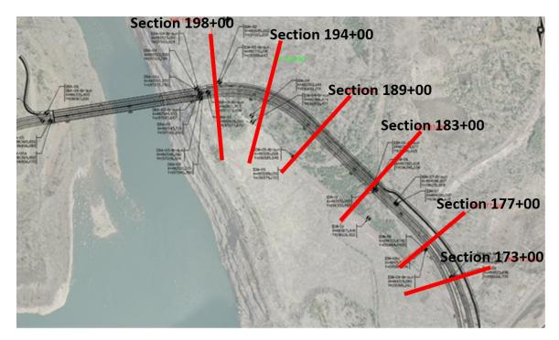
Figure 8 – Aerial image of the bridge alignment prior to construction, showing sections used for *UDEC* modeling.
