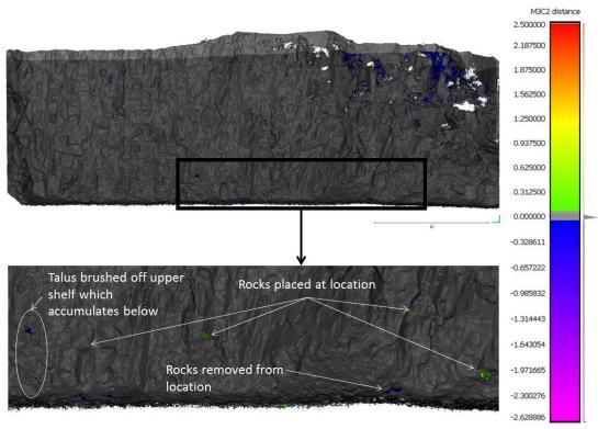
Figure 10: Change detection map of E-137-2 (Top) with the bottom image showing the locations on the slope where modifications were made between surveys. The degree and distribution of change is indicated in the histogram to the right of the colour scale. Units on the scale bar are reported in meters with the 5cm LOD shown in grey. The blocks moved on the slope range in volume from 10-45cm<sup>3</sup>.
