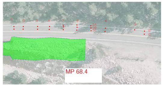
Figure 8. Plan View of Typical Grid Pattern Drilling.
