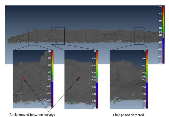
Figure 8: Change detection map highlighting the locations of rocks moved between surveys. Scale bar units are in meters; limit of detection +/- 10cm as shown by grey colour.
