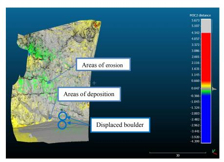
Figure 7: Change detection showing displaced rock from slope and erosion/deposition of soil
