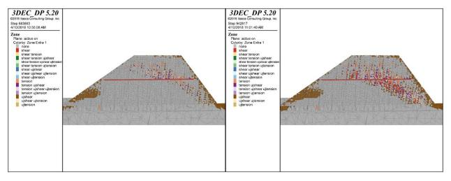
Figure 18 – Zones with various material failure behavior for the cross section at the bridge abutment for a factor of safety of 1.5 (left) and 1.8 (right).
