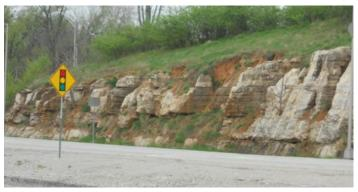
slabs and can exhibit problematic shrink and swell characteristics. For the tunnel, the Louisville Limestone presents several potential problems, most associated with the discontinuities such as solution enlarged joints (both horizontal and vertical), solutioning along bedding planes, voids, and sinkholes. The Louisville Limestone can also produce significant groundwater flows after rain events. Water flow is largely along open joints, fractures and bedding planes.
