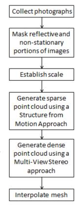
Figure 2: Processing workflow within Agisoft Photoscan Pro, Version 1.2.4
