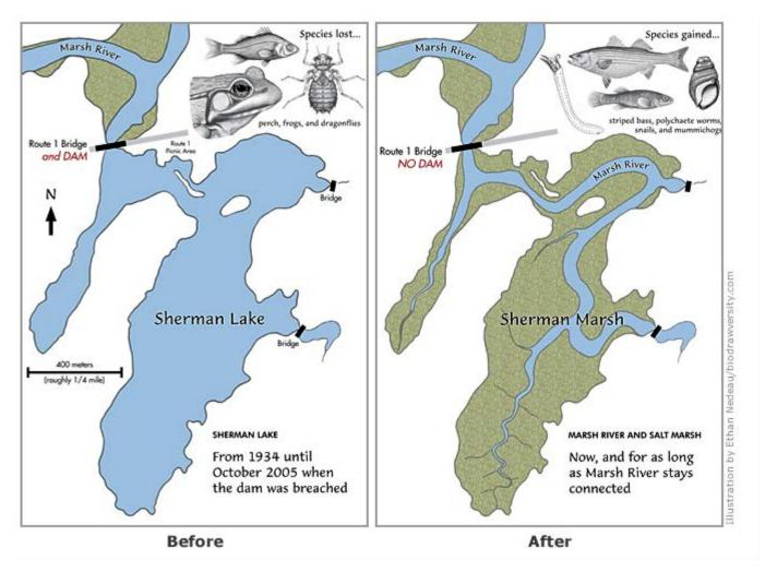
Figure 8. Configuration of Sherman Lake and Sherman Marsh before and after the dam breach and restoration.
