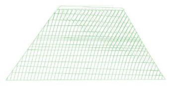
Figure 12 – Exaggerated (100x) deformed shape (in green) compared to the original shape (in grey), illustrating the nature of the flexural toppling mechanism.
