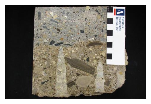
Figure 9 – saw cut and lapped pavement section showing many dark and angular igneous rock particles within the wear-course topping, a few were also noted in the base layer.
