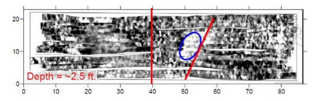
Figure 9. GPR Depth Slice from Site 1.
