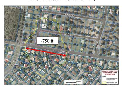
Figure 5 Failure of ~20ft to 30ft High Pillars at ~330ft to 500 ft. Depth With 4.6ft. of Subsidence in Ipswich, QLD, AUS, QLD Dept. of Mines and Energy Website
