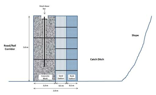
Figure 4 – Cross-Section through Modular Rockfall Protection Wall
