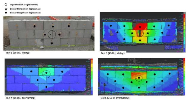
Figure 9 – Comparison of horizontal displacements for selected tests (colour scales differ)
