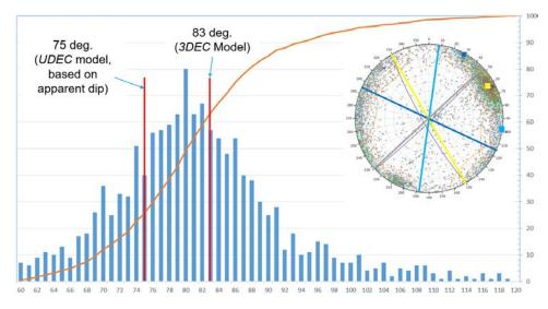
Figure 13 – Dip histogram for Joint Set 2.
