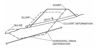
Figure 8 – Illustration of potential damage in embankments
