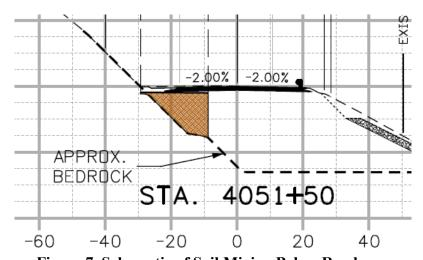
Figure 7. Schematic of Soil Mixing Below Roadway.
