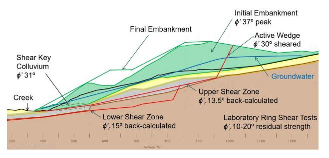
Figure 4 – Parametric Stability Analyses (Cougar Creek Slide)
