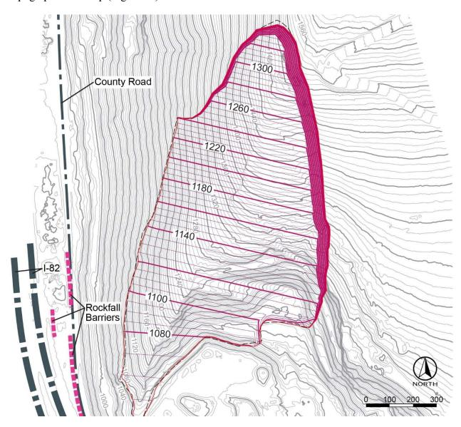
Figure 11 – Interpreted Geometry of Landslide Shear Zone
