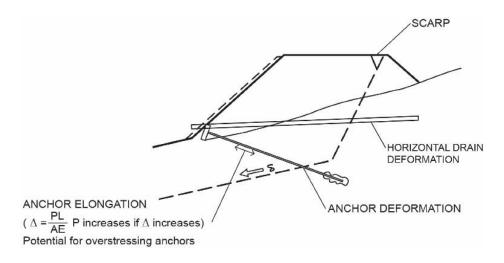
Figure 10 – Illustration of potential damage in ground anchors
