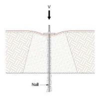
Figure 8 - Nail-Direction Load Characterized by In-Soil Punch Test
