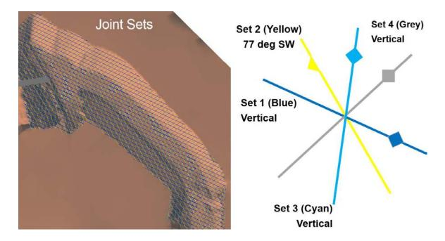
Figure 7 – Average joint set orientations intersected with the isthmus.
