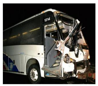
**Figure 8** – Direct icefall impact damage to bus near Terrace, British Columbia, courtesy of Terrace Daily Online, February 5, 2011.
