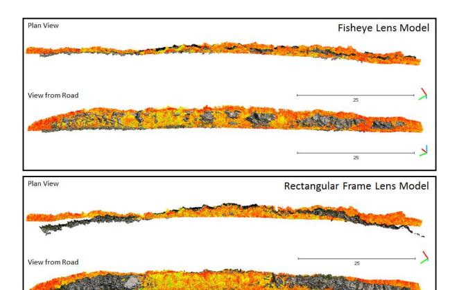
Figure 5: (Top) Photogrammetry model produced using a 10.5mm fisheye lens shown in true colour. (Bottom) Photogrammetry model produced using a 35mm rectangular frame lens shown in true colour. An aligned LiDAR model is shown in both images in orange and yellow.
