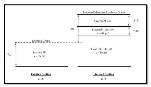
Figure 5: Compensating Fill Embankment Concept
