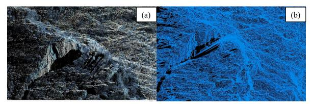
Figure 5 – Images of Point Cloud (a) and the Generated Mesh (b)
