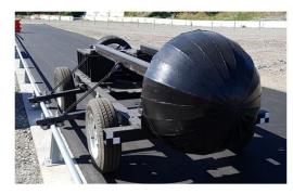
Figure 7 – Test bogey and guide rail system
