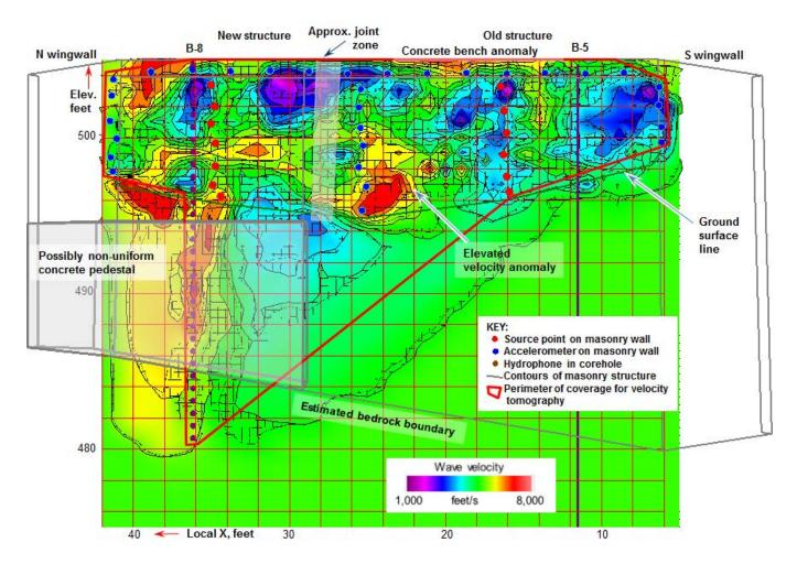
Figure 5 – Tomograph combined with the volumetric contour image of velocity distribution reconstructed along Abutment 1.
