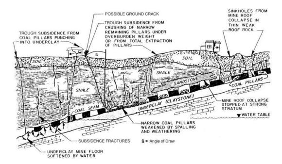
Figure 2 Types of Subsidence and Subsurface Conditions (Modified from Bruhn et al, 1978)
