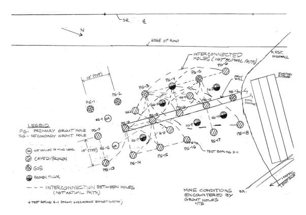
Figure 24 Field Mark-Up Showing Conditions Encountered and Interconnection of Workings
