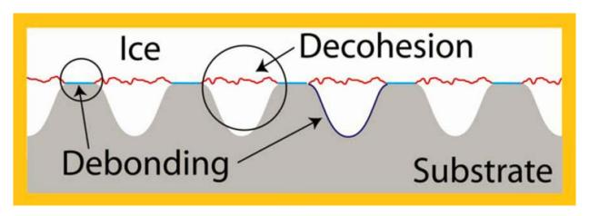
**Figure 6** – Idealized graphic of cohesion vs. adhesion loss along an ice-rock interface. Image adapted from Fortin & Perron (5)
