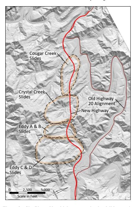
Figure 2 – Site Plan – New highway crossing landslide terrain
