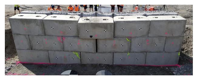
Figure 12 – Test Wall B following Test 6 (overturning, 750 kJ); steel fibre-reinforced concrete blocks
