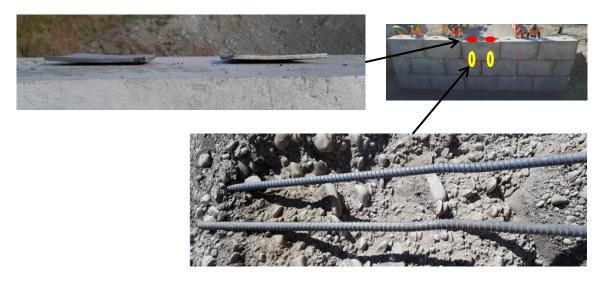
Figure 13 – Damage to steel bars and plates following Test 5 (2 x 250 kJ, overturning)
