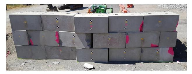
Figure 11 – Test Wall A following Test 3 (sliding, 750 kJ); plain concrete blocks
