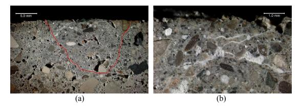
Figure 10 – anomalous paste 'nodule' (red outline) near the pavement surface which lacks fine air voids under 5x mag (a) fine sub-horizontal microcracking within the nodule highlighted by white secondary deposits under 25x mag (b)
