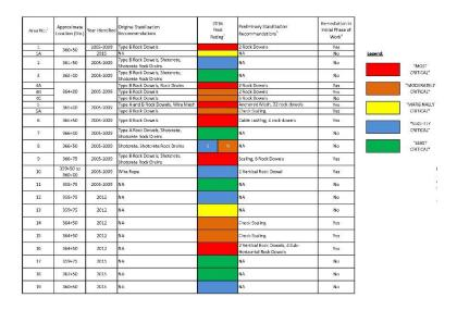
Figure 8 – Final Rock Slope Remediation Area Assessment
