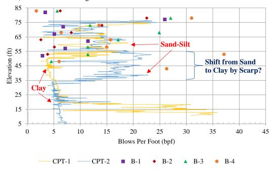
Figure 7 – Standard Penetration Test (SPT N<sub>60</sub>)
