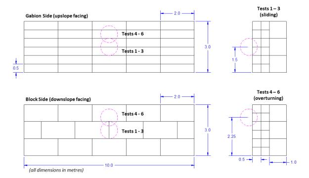
Figure 5 – Test impact locations for sliding and overturning failure modes
