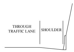
CUT SLOPE AT EDGE OF PAVED SHOULDER WITH BARRIER
