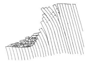
Figure 6 – Examples of rock movement caused by flexural toppling (Hittinger & Goodman, 1978).
