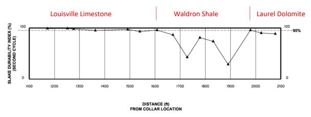
KYTC GEOTECHNICAL MANUAL DURABLE SHALE ≥ 95 NONDURABLE SHALE ≤ 95
