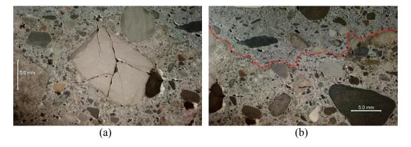
Figure 11 – cracking within soft dolostone coarse aggregate particle within base layer concrete under 5x mag (a) and sub-horizontal cracking within base concrete paste near the contact with the wear-course (red line) under 5x mag (b)
