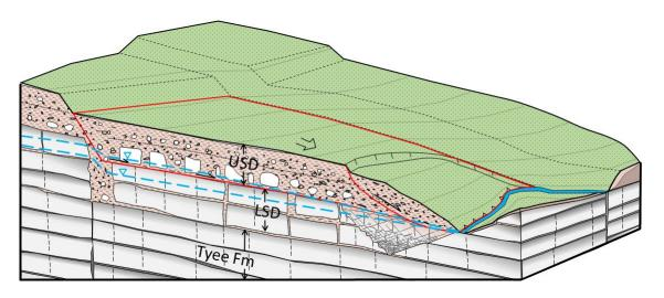
Figure 3 – Landslide Stratigraphy
