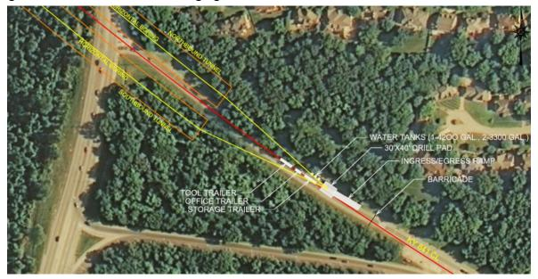
The North Bound boring was the first boring drilled. We used an LM-75 skid mounted underground drill rig to complete the North Bound boring. The South Bound and Pillar borings were drilled using an LM-90 skid mounted underground drill rig. The drill rigs were powered by Caterpillar generators which were quiet enough you could easily talk with a normal volume
