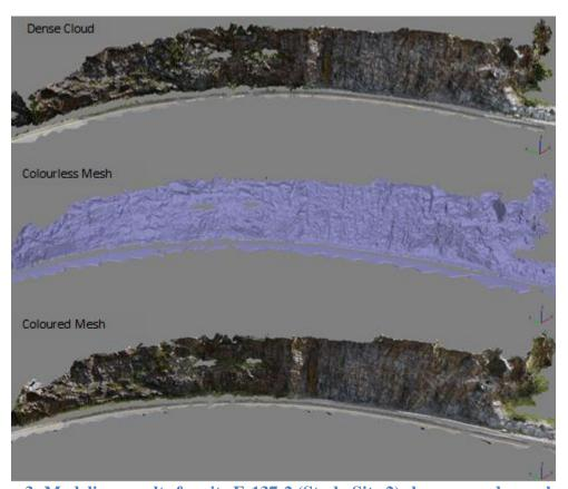
Figure 3: Modeling results for site E-137-2 (Study Site 2) shown as a dense cloud, a colourless mesh, and a coloured mesh.
