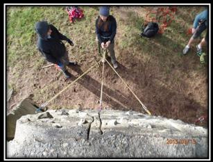
Figure 11: Evaluate slope for available anchors for safety and rappel lines. In the left photo the technician is using 1-inch webbing around a tree for a rappel anchor. Right photo, technician is demonstrating a 3-point anchor using mechanical camming devices.
