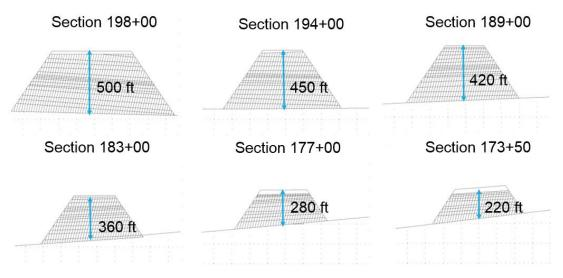
Figure 9 – Cross-sections modeled using *UDEC* (sections looking toward bridge, for joints dipping 75 degrees left).
