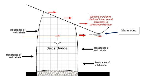
Figure 8 Lateral Dilation Mechanism for Horizontal Movement (Commonwealth of Australia, 2014)
