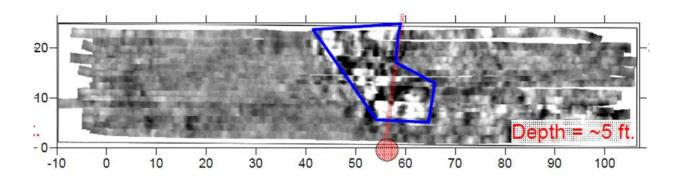
Figure 11. 5-Ft GPR Depth Slice from Site 2.
