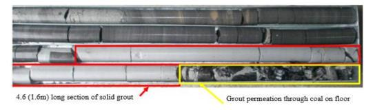
Figure 25 View of Grout Recovered from Cored Verification Hole
