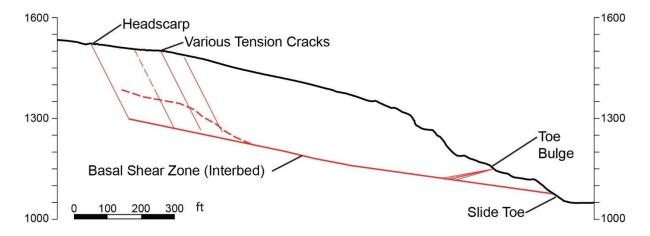
Figure 12: Landslide Cross Section
