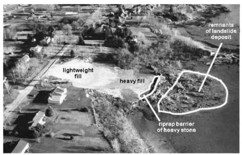
Figure 8. Oblique aerial image of remediated 1996 landslide site, looking roughly east (from Berry and others, 1997).
