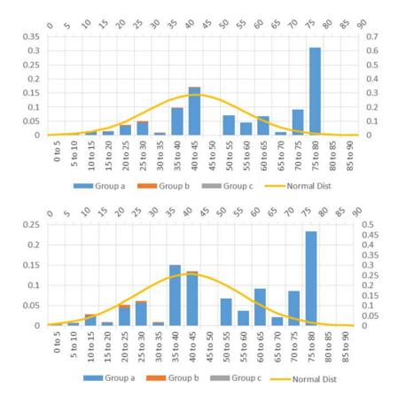
Figure 10 – Joint frictional strength properties (top) and bedding frictional strength properties (bottom).
