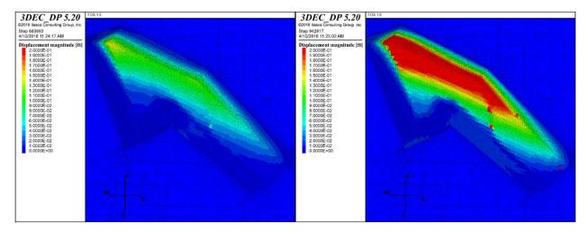
Figure 15 – Predicted surface displacements at equilibrium for a safety factor of 1.5 (left) and 1.8 (right).
