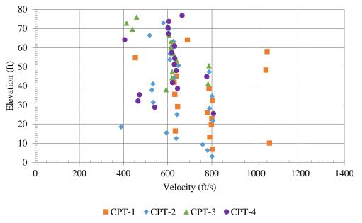
Figure 8 – Shear Wave Velocity (Vs)
