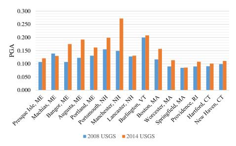
Figure 2 – USGS Hazards Mapping PGA (2% in 50 Years)
