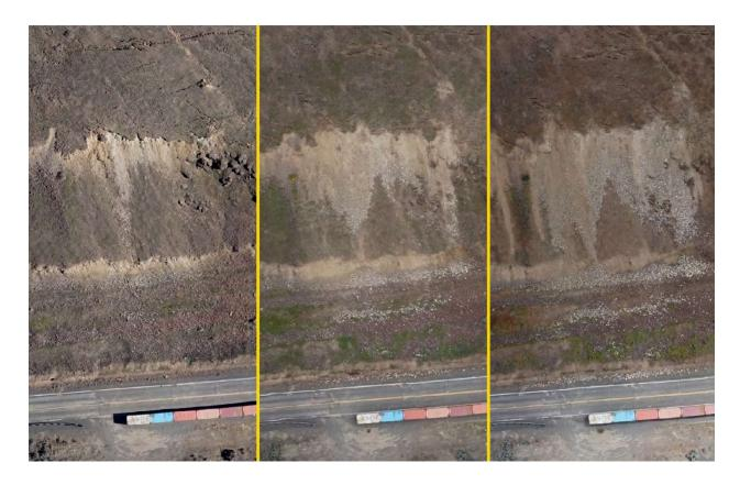
Figure 9 – Raveling Along West Flank of Landslide, Producing Rockfall (February 26, April 11 and May 9, 2018)
