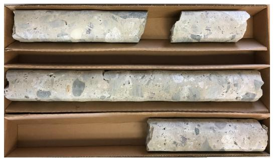
Figure 10. Recovered Core Samples of Soil Cement.
