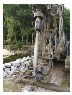
Figure 7 – Drill Rig and Robit Hammer
