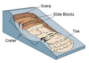
Figure 3. Cartoon illustration of a rotational landslide (modified from Highland and Bobrowsky, 2008). The 1996 Rockland landslide is an excellent example of this landslide morphology, also visible in Figures 4 and 5. A slide is considered "retrogressive" if it continues to migrate back into the slope after the initial failure. Retrogression usually ceases when enough failed material accumulates to buttress the slope.
