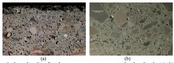
Figure 6 – lapped section of top layer or wear-course concrete showing abundant (sub) spherical air voids within its paste under 10x mag (a) and comparison to a modern concrete with purposeful air entrainment under 10x mag (b)
