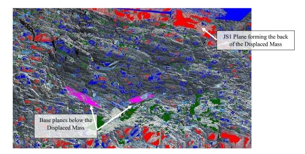
Figure 10 – Patches (Pink) Representing Base Planes in Beneath the Displaced Mass
