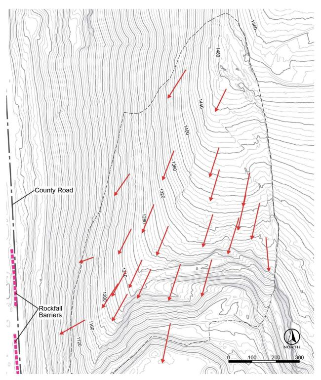
Figure 5 – Landslide Horizontal Movement Vector Directions
