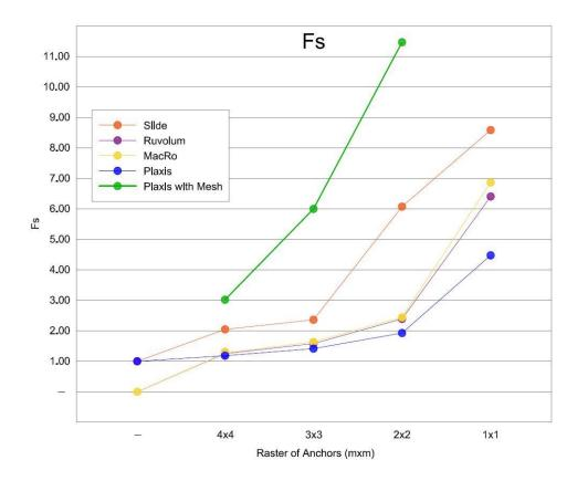
Figure 12 - Results Showing the Variation of Fs Versus Nail Spacing as a Function of Method of Analysis
