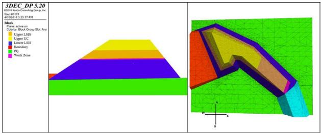
Figure 3 – Geologic units in section view (left) and in plan view (right).
