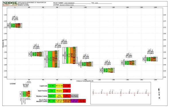
Figure 5 – NDDOT gINT Fence Color Sheet with boreholes plotted to horizontal and vertical (elevation) scale. Note that LSS-3 and LSS-4 have been offset so there is not horizontal overlap.
