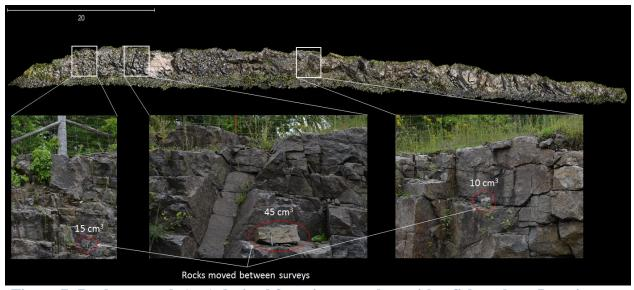
Figure 7: Rock cut mesh (top) derived from images taken with a fisheye lens. Inset images show the locations and approximate volumes of rocks being moved between surveys.
