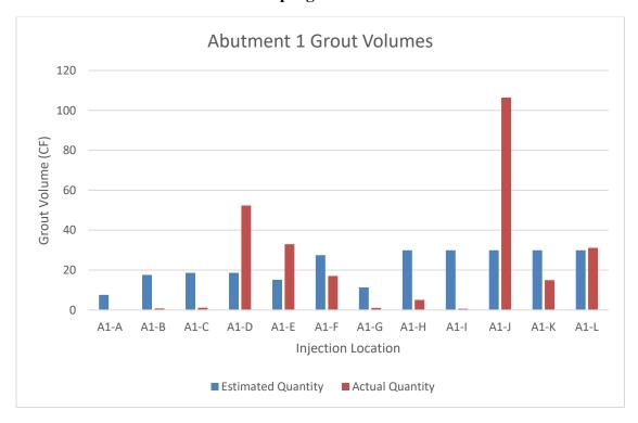
Figure 10 – Total volumes of grout placed at each injection point in Abutment 1.
