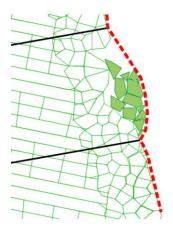
Figure 5 – Deformed Mesh with Forces Characterized by In-Isolation Punch Test
