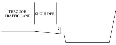
CUT SLOPE WITH DROP ZONE AND BARRIER
