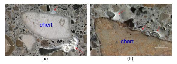
Figure 12 – chert fine aggregate particles undergoing minor ASR within the wear-course concrete, red arrows indicate proximal deposits of secondary bright white ASR gel under 25x mag (a) and 50x mag (b)
