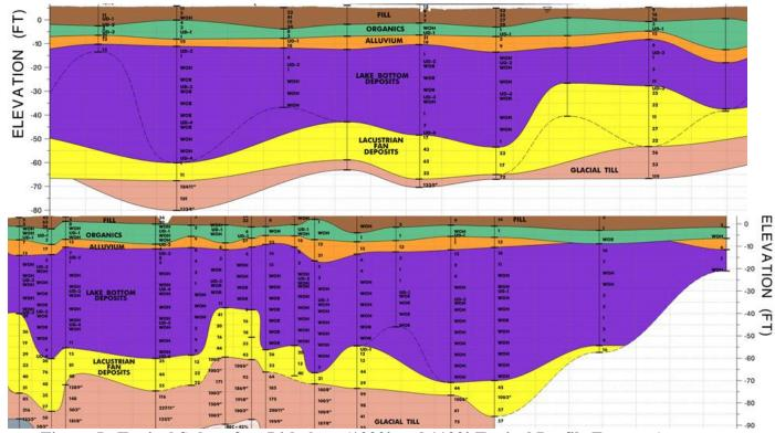
Figure 5– Typical Subsurface Lithology (1000' and 1100' Typical Profile Excerpts)
