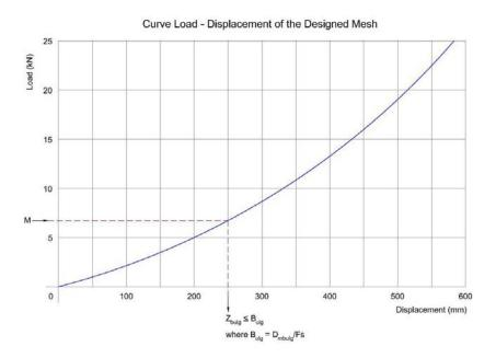
Figure 7 - Example of a load-displacement curve used for the design of the mesh at the Serviceability Limit State
