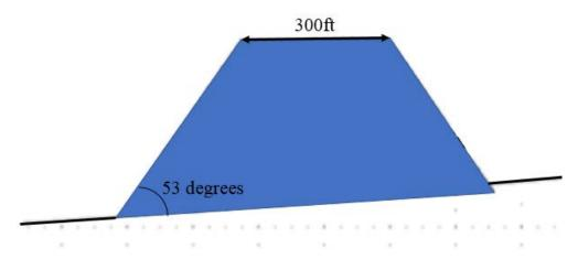
Figure 2 – Isthmus cross-section at Station 183+00.
