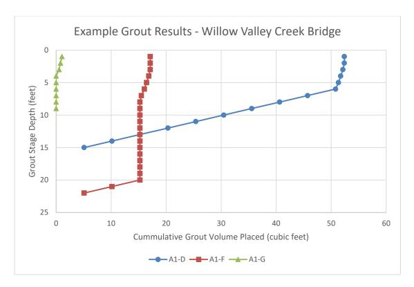
Figure 9 – Example grouting logs from Abutment 1. Grouting proceeded from Hole A1-D, then A1-F, and last, A1-G. Note that total grout volume decreases as the program progresses.
