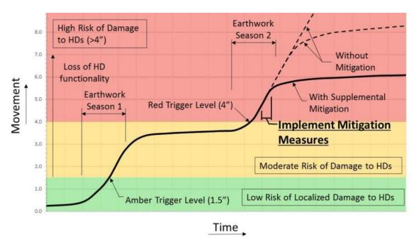
Figure 14 – Illustration of potential movement trends and stages of Observational Method for embankments, including trigger criteria and increased level of monitoring, possibly leading to decision to implement a supplemental mitigation
