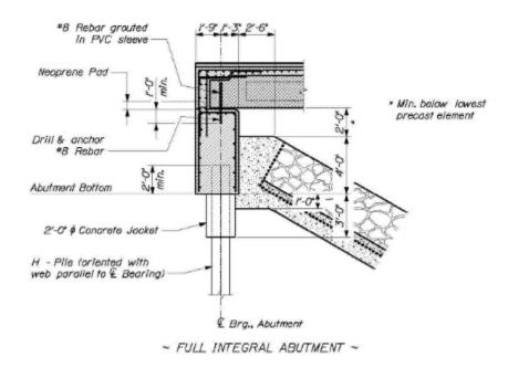
Figure 5 – Integral Abutment Detail
