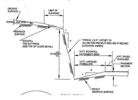
Figure 4 – Design Rock Slope and Catchment Area Geometry
