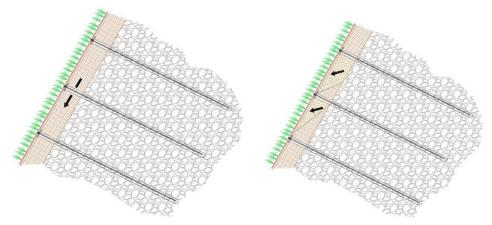
Figure 3 – (a) Slope-Parallel Instabilities and (b) Between-Nail Instabilities
