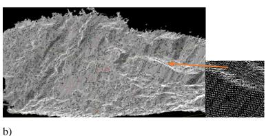
Figure 3: a) point cloud from sfm photogrammetry and b) DSM made from triangulated mesh surface.
