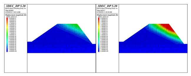
Figure 17 – Model displacements for the cross section at the bridge abutment for a factor of safety of 1.5 (left) and 1.8 (right)
