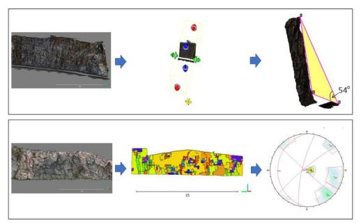
Figure 6: (Top) Cross section of a point cloud used to estimate the Crest Angle. (Bottom) Extraction of joint orientation data from a point cloud to a stereonet.
