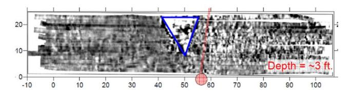
Figure 10. 3-Ft GPR Depth Slice from Site 2.
