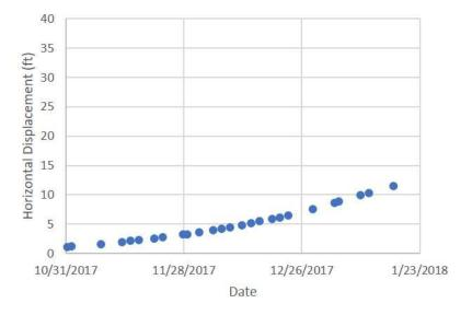
Figure 6 – Landslide Horizontal Movement (RTK, October 2017 to mid-January 2018)
