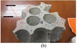
Figure 2 – pre-submittal photos of intact concrete pavement segment (a) and previously-cored segment (b) (photos supplied by the ACPA)
