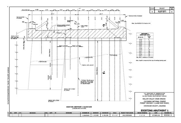
Figure 8 – Abutment 1 (East) grouting plan.
