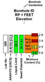
Figure 3 – Legend depicting a typical borehole on the NDDOT gINT Fence Color Sheet.
