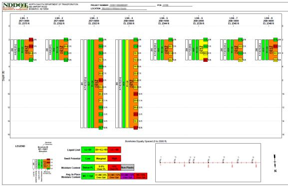
Figure 6 – NDDOT gINT Fence Color Sheet with boreholes plotted equally-spaced and with a depth scale.
