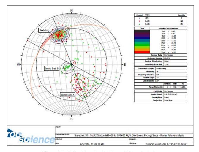
Figure 8 Rock Cut Slope No. 2 – Planar Failure Analysis
