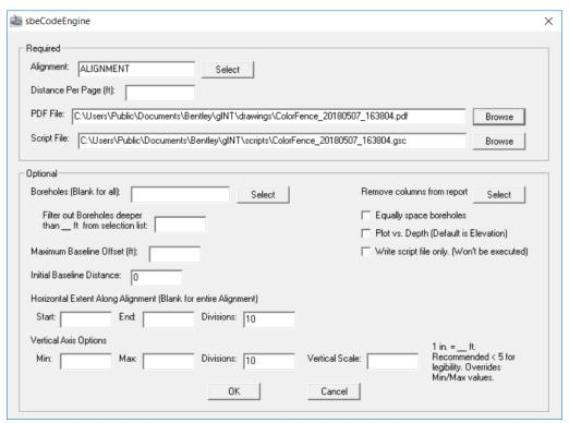
Figure 4 – Interface for the Add-In to create the NDDOT gINT Fence Color Sheet.
