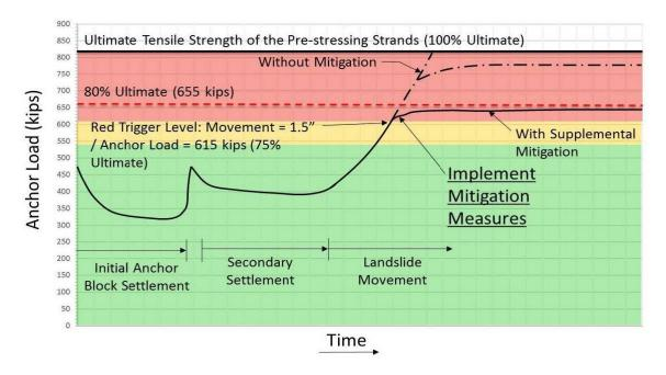
Figure 15 – Illustration of potential movement trends and stages of Observational Method for ground anchors to stabilize embankments, including trigger criteria and increased level of monitoring, possibly leading to decision to implement a supplemental mitigation
