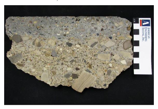
Figure 3 – saw cut and lapped cross-sectional profile of Bellefontaine pavement sample. Note the two-layer construction is evident by both paste coloration and aggregate sizing
