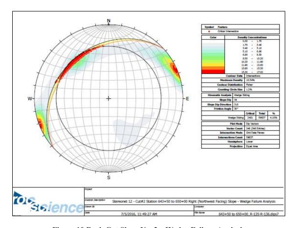
Figure 10 Rock Cut Slope No. 2 – Wedge Failure Analysis
