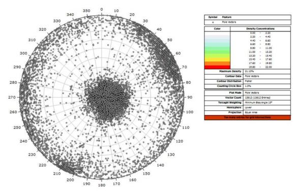
Figure 4 – Lower hemisphere stereonet of all joint and bedding orientations for the isthmus rocks.
