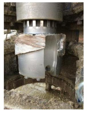
Figure 8 – Robit Air Hammer Tip (side)
