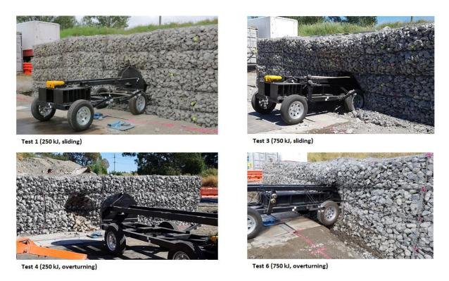
Figure 10 - Comparison of bogey penetration and gabion deformation for selected tests
