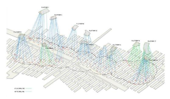
Figure 23 Example of Grouting Using Designated Drilling Pads (Kingsland, et al., 2012)
