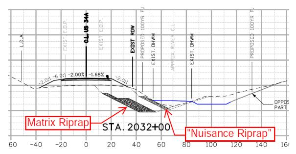
Figure 6. Schematic of Matrix Riprap with Nuisance Riprap.
