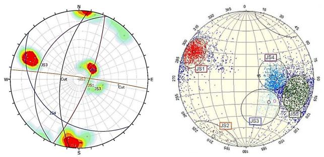
Figure 7 – Joint Set Groupings: Poles of Hand Measurements (left) and Poles of Split-FX® Patches (right)
