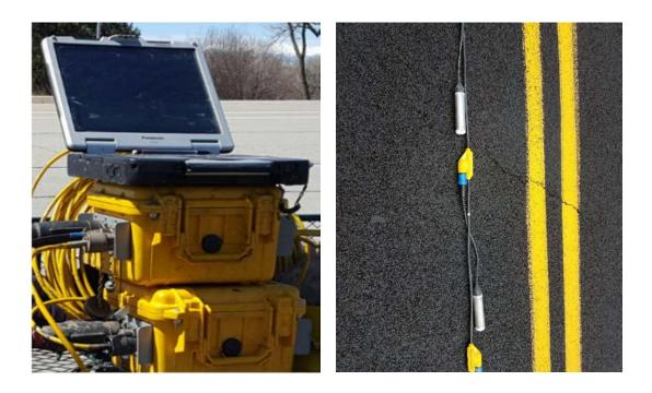
Figure 6: Left – Seismograph and Laptop. Right – Typical Geophone Configuration.
