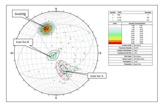
Figure 7 Rock Cut Slope No. 2 – Discontinuity Contour Plot
