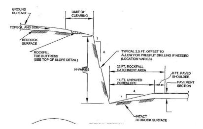
Figure 5 – Design Rock Slope and Catchment Area Geometry
