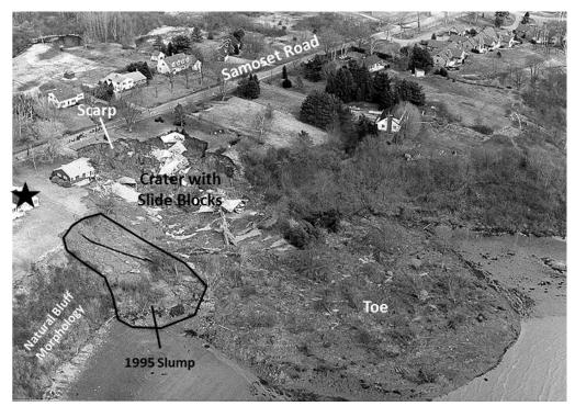
Figure 7. Oblique aerial view of the 1995 slump and 1996 landslide, looking east.
