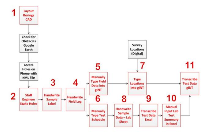
Figure 2 – Typical Workflow for Consultants Performing Subsurface Investigations
