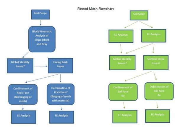
Figure 13 – Proposed Flowchart for the Design of Pinned Drapery Systems [5]
