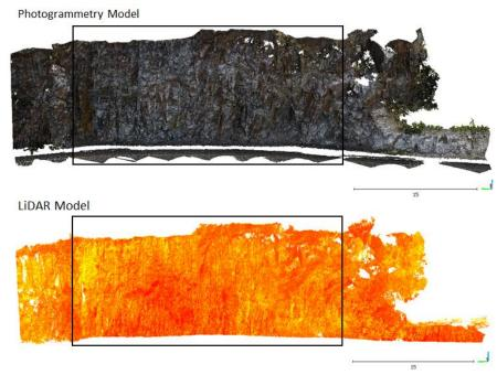
Figure 9: Photogrammetry model (top) and LiDAR model (bottom). The section of the face where modifications were made between surveys is outlined by the black box.
