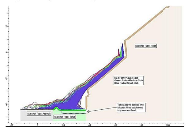
Figure 14 - Filled Catchment Configuration and Rock Paths
