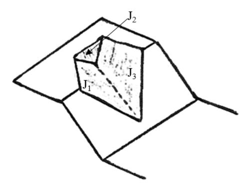
Figure 4: Sketch showing a rockfall void and bounding surfaces (J<sub>1</sub>, J<sub>2</sub>, and J<sub>3</sub>).
