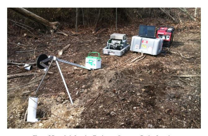
Figure 5 Downhole Logging Equipment Setup at a Boring Location
