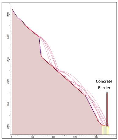
Figure 16: RocFall trajectories down the critical cross section (profile K).
