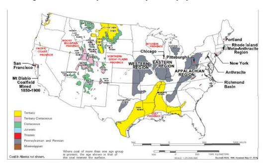
Figure 1 Coal Bearing Areas of The Lower 48 States Note Underground Coal Mining Has Also Occurred in Alaska. (Modified From USGS, 1996).
