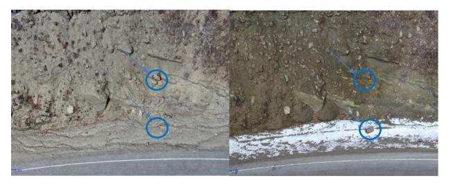
Figure 8: (a) November 2017 image showing rock prior to fall (b) January 2018 image showing rock following fall
