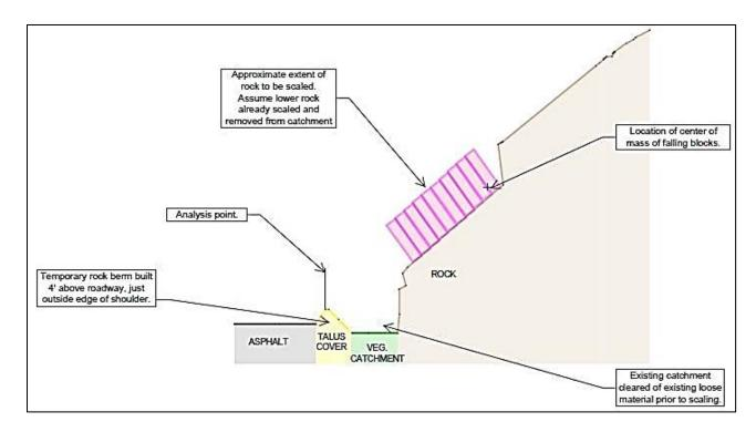
Figure 13 - Initial Slope Configuration for Rockfall Evaluation During Scaling
