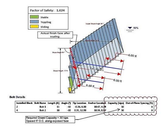
Figure 11 – 50 Percent Water Pressure Model Evaluated in RocTopple with Reinforcement
