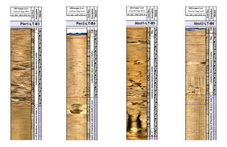
Figure 4 – Example downhole image showing void space within the mortared cut-stone masonry B3-B4-B5-B6. Old section (B3 and B5) versus newer section (B4 and B6).
