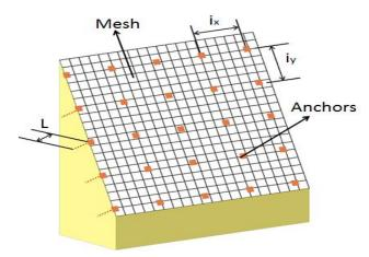
Figure 1 - Pinned drapery system: the intervention is composed of a steel wire mesh and a pattern of anchors (L = length of the anchors;  $i_x$  and  $i_y = distance$  between the anchors, respectively horizontally and vertically).
