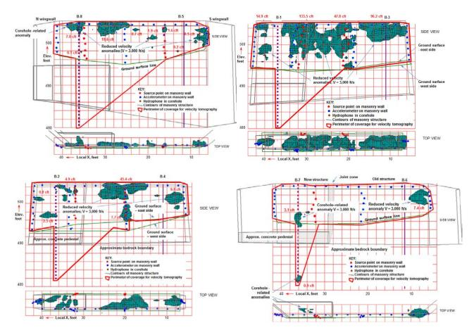
Figure 6 – Tomographic representation of possible compromised structural integrity volumes for Abutment 1 (upper left), Pier 1 (upper right), Pier 2 (lower left) and Abutment 2 (lower right)
